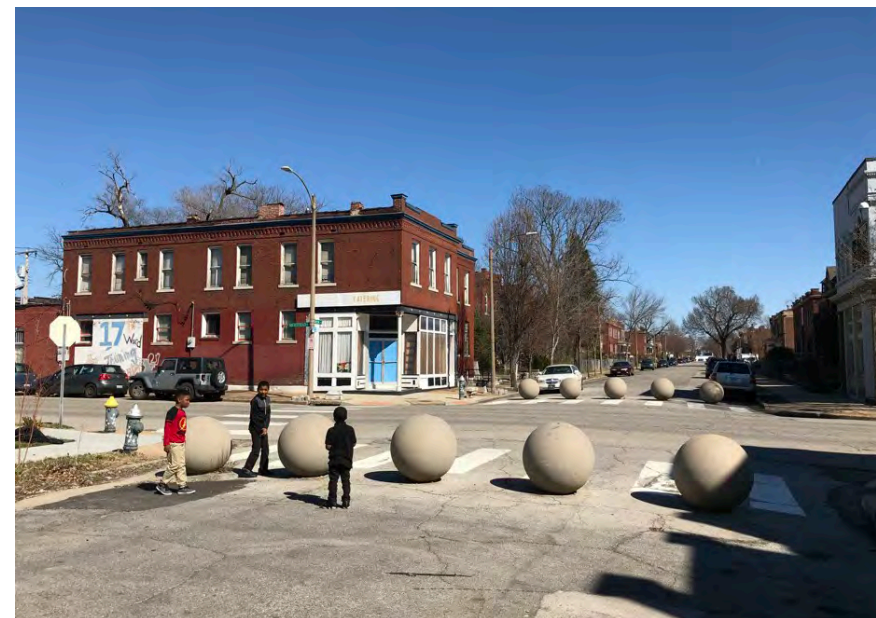
This example shows how existing streets and intersections can quickly be transformed into pedestrian gateways using more permanent bollards.
