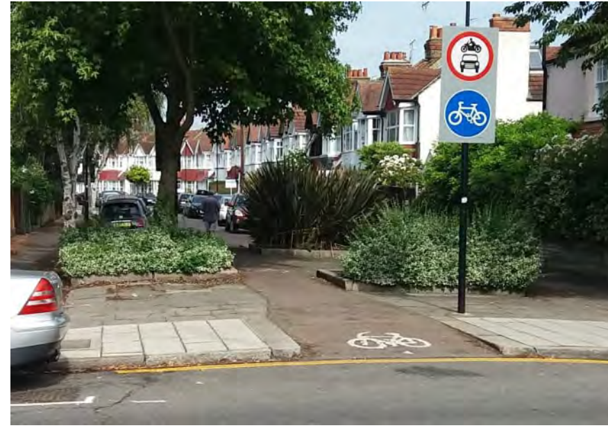
A fully-constructed, permanent pedestrian gateway (as shown here) can be viewed as both a passageway and a small pocket park. This example shows how planting, pavers, and signage work together to make this pedestrian gateway feel like a welcoming space.
