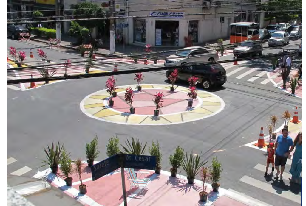
Painted bumpouts and roundabouts with planters, bollards, or other barriers are effective substitutes for the fully constructed version. These could be temporary solutions that would be upgraded to more permanent fixtures over time.
